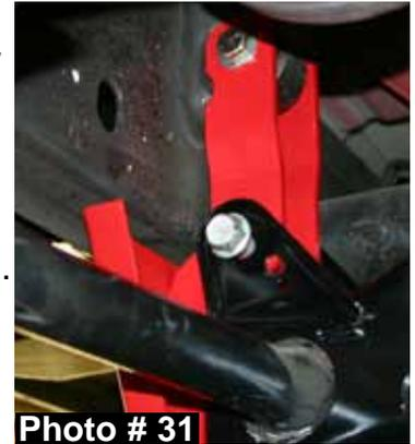
41. **6" Lift:** Install the new Skyjacker torsion bar drop brackets to the OEM torsion bar cross member frame mounts using the supplied 9/16" x 4" bolts, 9/16" SAE washers, & 9/16" nuts. Reinstall the OEM torsion bars, OEM torsion bar keys, & OEM torsion bar cross member using the OEM hardware & 21mm socket. (See Photo # 31) **Note:** Be sure to install the OEM adjuster bolts to the same length as OEM when removed in Step # 5.
