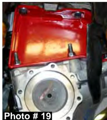
25. Apply thread locking compound to the OEM hardware & reattach the OEM front drive shaft using a 11mm socket. **Note:** Be sure to reinstall in the exact same position with the marks made to the OEM u-joint & yoke from Step # 15. Some models, may require the OEM transmission pan flange to be slightly ground for clearance of the OEM front drive shaft. (See Arrow in Photo # 20)
