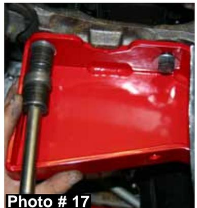
23. Support the OEM front differential & attach the front differential to the new Skyjacker passenger side differential bracket using the supplied 12mm x 40mm bolts, 7/16" USSW washers, 12mm nuts, 18mm socket, & 19mm socket. (See Photo # 18)
