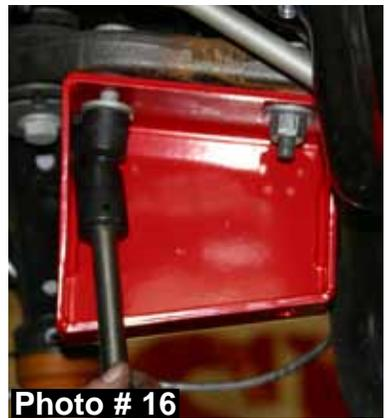
22. Install the new Skyjacker driver side differential bracket to the OEM mount using the supplied 12mm x 40mm bolts, 12mm x 90mm bolt, 7/16" USSW washers, 18mm socket, & 19mm socket. The new driver side differential bracket will install with the open end to the outside & the longer end toward the front of the vehicle. (See Photo # 17)
