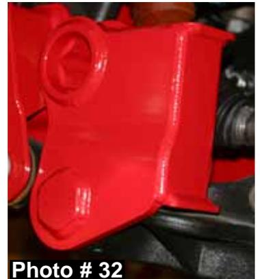
42. **7" Lift:** Install the new Skyjacker raised torsion bar brackets by aligning the hex of the torsion bar brackets with the hex of the lower a-arms, completely seating the brackets with the lower a-arms. (See Photo # 32) Reinstall the OEM torsion bars, OEM torsion bar keys, & OEM torsion bar cross member using the OEM hardware & 21mm socket. **Note:** Be sure to install the OEM adjuster bolts to the same length as OEM when removed in Step # 5.
