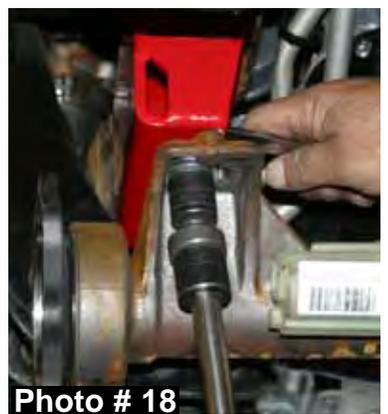
26. Attach the electrical connector to the the OEM front differential actuator & attach the wire to the top of the OEM front differential using the supplied plastic tie.
