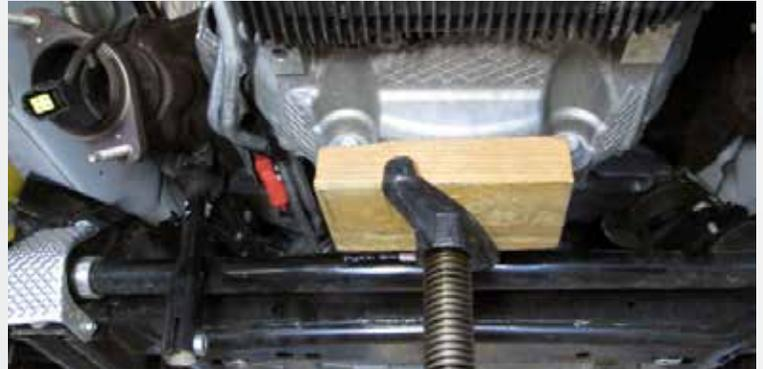
Safely support engine for removal and install of motor mounts.
