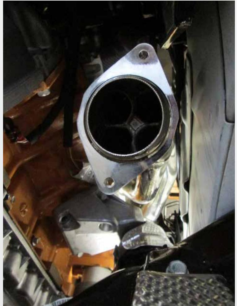
Install BBK headers with supplied gaskets and hardware making to use dipstick bolt and nut. Re-attach alternator brace and install motor mount. Then install factory head pipes. Install factory plastic shields and start vehicle checking for any leaks. Recommended to re-torque all header fasteners the following day after a couple heat cycles.
