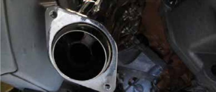
Install BBK headers using supplied hardware and gasket with 12mm socket/wrench. Re-install motor mount and steering shaft.
