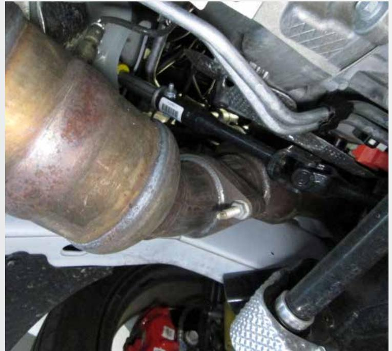
Disconnect O<sup>2</sup> sensor plugs and then remove factory head pipe using 16mm socket.
