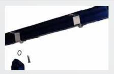
Install the mounting tabs onto the bottom of the BBK rails by placing a washer over the threads of each of the supplied ½"-20x 3/8" (shorter button head) Allen bolts and placing the bolt through the round hole (not the slot) in each bracket.
