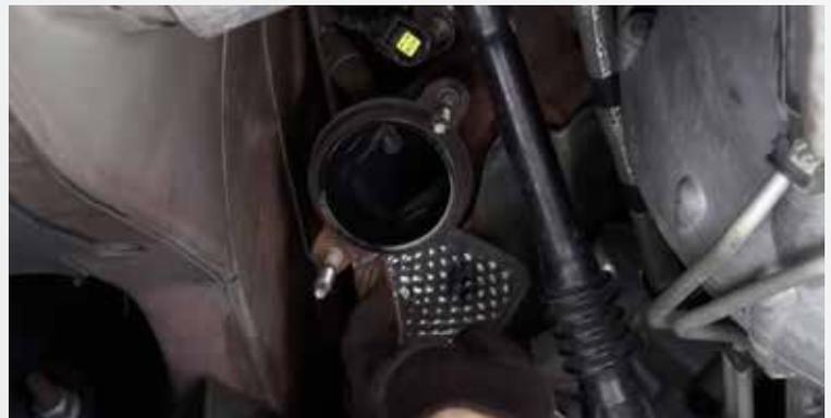
Remove the heat shields from the motor mounts and the factory exhaust manifolds.
