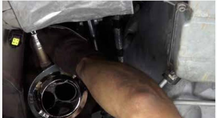
Install the BBK headers by sliding the slots onto the started bolts (over the gaskets) then inserting and tightening all of the supplied header bolts.
