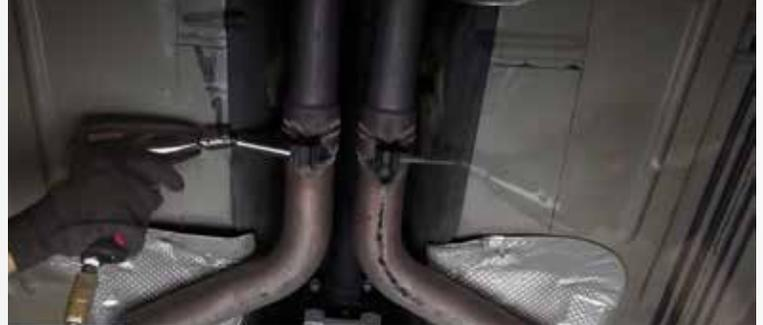
Remove the nuts that attach the H-Pipe to the factory manifolds.
