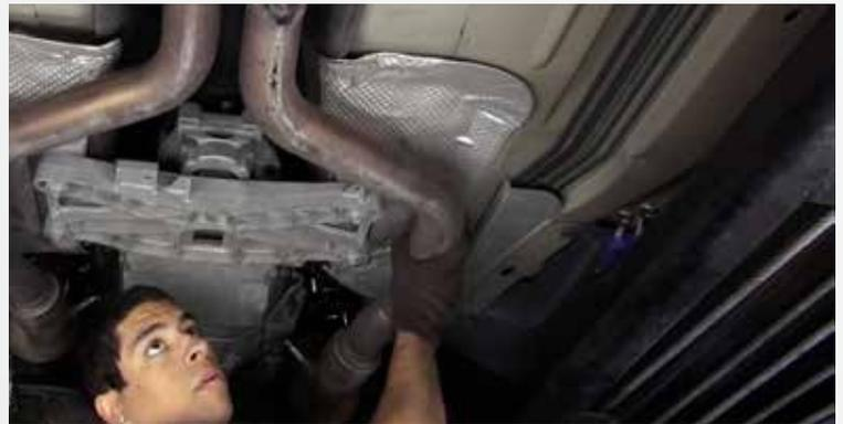
Push the H-Pipe forward to meet up with the BBK Headers and tighten the collector flanges using the supplied washers and nuts. Then tighten the H-Pipe clamps.
