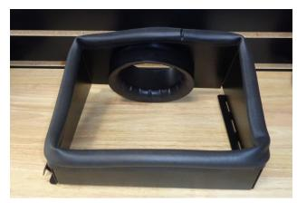
10. Attach the gasket (4) to the heat shield. Firmly press the gasket onto the heat shield, gradually working your way around. When you return to the starting point, use metal-cutting shears to trim the gasket to length.
