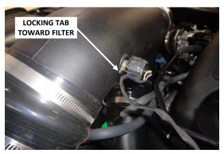
19. Carefully push the inlet air temperature sensor into the grommet and point the locking tab toward the air filter. (Moistening the hole with soapy water will ease insertion.) Reinstall the sensor plug and verify that the connection is secure.
