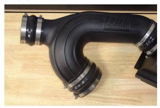
14. Slip the other 2 large screw clamps (11) onto the 4-1/2" - 4" coupler (14). Slip the 2 small screw clamps (16) onto the 3-1/2" - 3" coupler (15). Push the large end of each coupler onto the intake tube. Snug – do not tighten – only the tube clamps at this time. (Leave the other clamps loose.)
