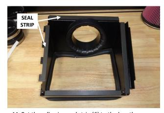
11. Cut the adhesive seal strip (6) to the lengths required, and apply it to the four edges of the heat shield.
