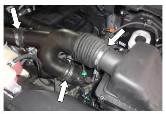
Loosen the screw clamps on the 3 ends of the air intake duct.
