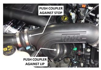
18. Push each coupler up against its stop on the turbo duct and tighten its turbo duct clamp. Then "center" the intake tube between the couplers (so that there are approximately equal amounts of tube inserted in each coupler), and tighten the three screw clamps on the intake tube.
