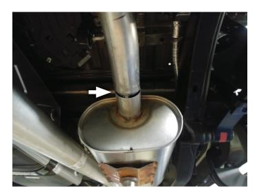
4. Dismount tailpipe from isolators (x3) then remove from vehicle.
