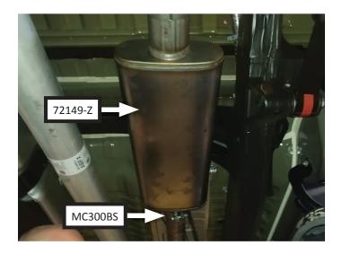
Place 3" clamp (MC300BS) onto muffler outlet. Route tailpipe (26741M) over rear axle then connect it to muffler. Insert wire hangers (x3) into factory isolators then tighten clamp just enough to allow for adjustment.
