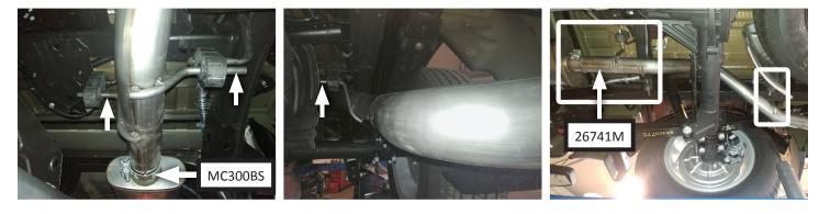
12. Place **tip (ST509B)** onto tailpipe. Tighten inlet to secure connection.
