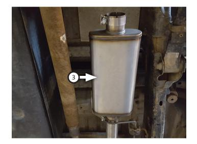
12. Place clamp (6) onto muffler outlet. Route tailpipe (4) over rear axle and connect it to muffler. Tighten clamp enough to allow for adjustment.
