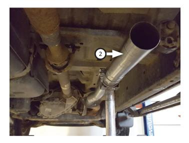
11. Place front hanger (7) onto muffler (3) then connect it to inlet/extension. Insert hanger into isolator and tighten clamp just enough to allow for adjustment.
