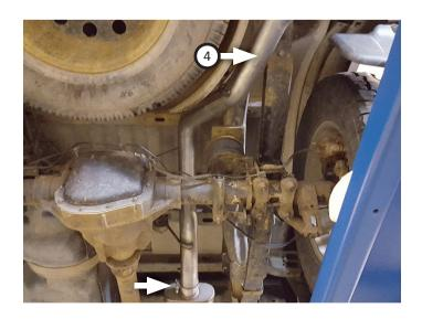
13. Connect **tip (5)** to tailpipe then tighten inlet to secure connection.
