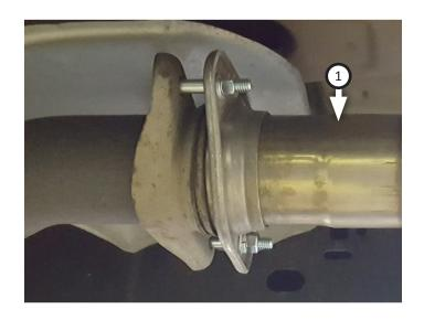
10. For applicable vehicles, place clamp (6) onto extension pipe (2) and connect it to inlet. Inlet pipe should be offset toward frame of vehicle.
