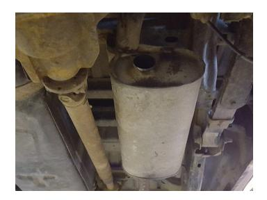
4. Dismount hanger from isolator and remove rear tailpipe section.
