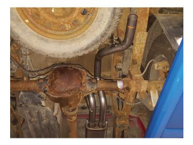
13. Secure rear frame mount (14) to vehicle using bolt (18) through frame, mount, flat washer (15), lock washer (16) and nut (17). Fit rubber hanger (13) onto end of hanger.
