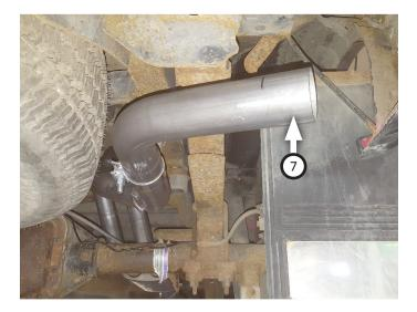
www.flowmastermufflers.com Technical Support (866) 464-6553 16. Connect **tips (x2) (8)** to side exit pipes and secure connections.
