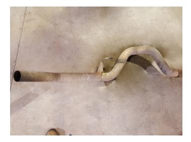
5. Remove bolts (x2) from flange at catalytic converter, disassemble wire hangers from isolators and remove muffler assembly from vehicle.
