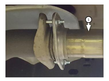
For applicable vehicles, place clamp (11) onto extension pipe (2) and connect it to inlet. Inlet pipe should be offset toward frame of vehicle.
