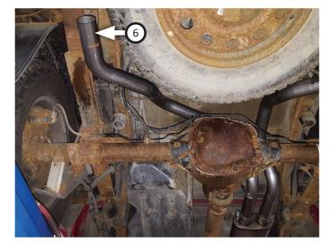
15. Place clamps (x2) (10) onto slip-fit of side exit pipes (x2)
