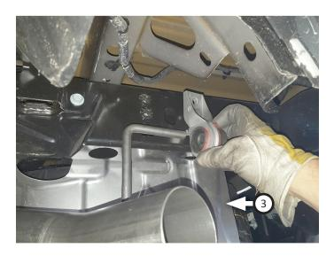
10. Place **tip (4)** onto tailpipe and tighten inlet. Rotate tailpipe and tip to desired distance from body or bumper, so angle cut on tip is properly positioned.
