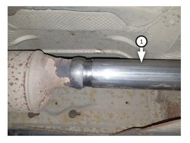
9. Place **clamp (5)** onto **muffler (2)** then connect it to inlet pipe. Tighten clamp just enough to allow for adjustment then place (x2) **clamps (6)** onto muffler outlets.
