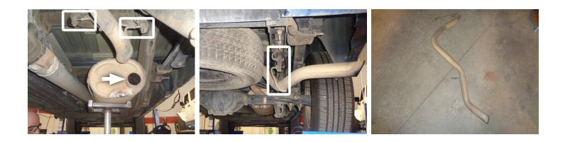
4. Disassemble wire hanger from isolator, loosen ball clamp and remove muffler section. Release tab to remove ball clamp from pipe and retain it for later use.
