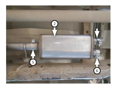
10. Slide **bracket (8)** onto **exit pipe (3)** wire hanger then connect it to muffler. Tighten clamp just enough to allow for adjustment.
