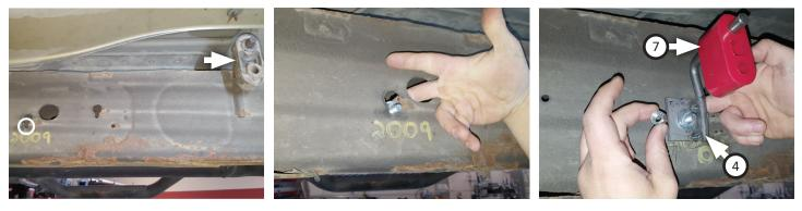
8. Place factory ball clamp (removed step 4) onto **inlet pipe (1)** then connect it to cat. converter. Insert wire hanger in isolator and tighten clamp enough to allow for adjustment.
