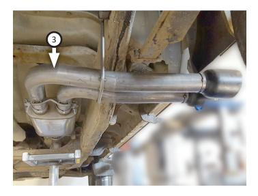
Adjust exit pipe until tips are desired distance from body, then lay bracket flat against vehicle rail and mark holes (x2). Rotate bracket away, drill marks with a ¼" drill bit then secure bracket to rail using (x2) **bolts (9)**.
