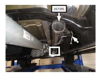
11. Place clamps (x3) (MC300BS) on muffler (8530572-266) inlet and outlets, then connect muffler to inlet pipe. Tighten clamp on muffler inlet just enough to allow for adjustment. Connect grounding wire to inlet pipe.
