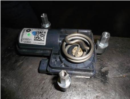
3) Place the actuator assembly against the bracket on the new Flowmaster tailpipe as shown in the first photo below, the center arm of the spring will be between the tabs on the bracket. Rotate the assembly so that the actuator motor is upright and until the spacers line up with the holes in the bracket. Install the included #10-32 x 3/8" Button Head Screws from the back of the bracket and into the spacers as shown in the third photo below. Tighten securely.
