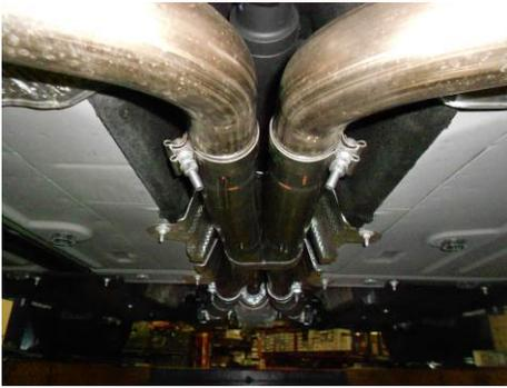
4) Begin the installation by placing a supplied 2-3/4" clamp onto each of the inlets of the Scavenger pipe **#26522S**. Then place the Scavenger pipe onto the back of the stock head pipes (the offset outlet pipe should be oriented to the right side). Level and center the assembly in the drive line tunnel and support with a stand. Tighten the two clamps enough to hold, but still allow for adjustment.
