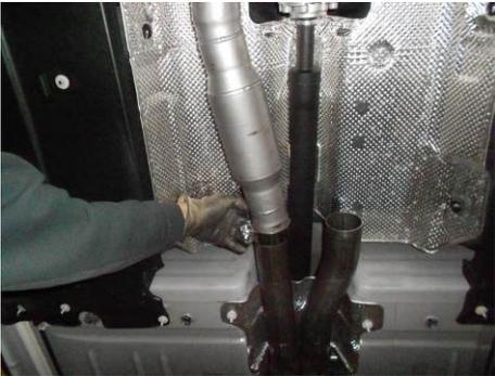
5) Place a supplied 3" clamp onto the inlet neck of both mufflers. Slide the mufflers onto the back of the Scavenger pipe assembly and support with stands. Level the mufflers and tighten the clamps enough to hold, but still allow for adjustment.
