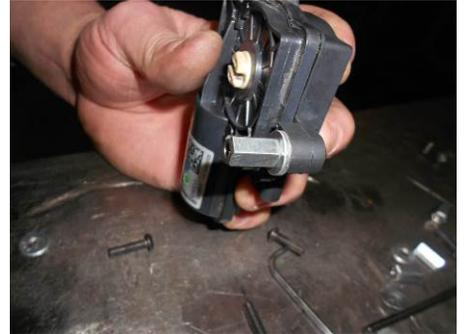
2) The actuator with the spacers and spring attached.
