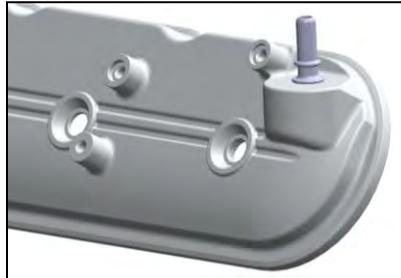
13. Remove the individual coils from the original bracket and install each onto the Holley valve covers. Torque coil bolts to 12 Nm (106 lb in).
