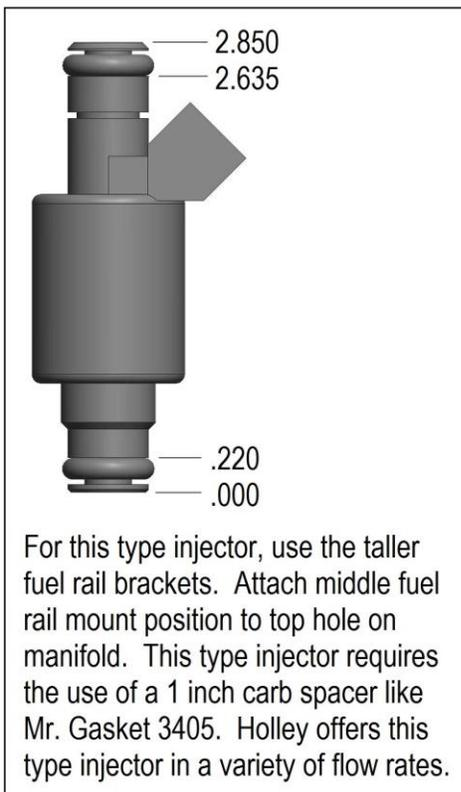
For this type injector, use the taller fuel rail brackets. Attach middle fuel rail mount position to top hole on manifold. This type injector requires the use of a 1 inch carb spacer like Mr. Gasket 3405. Holley offers this type injector in a variety of flow rates.
