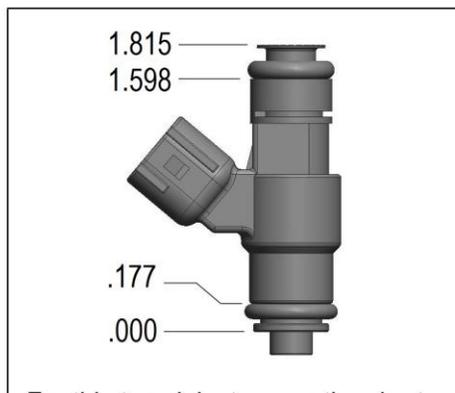
For this type injector, use the shorter fuel rail brackets. Attach middle fuel rail mount position to bottom hole on manifold. For this type injector, Holley offers 522-361S (1pc.) or 522-368S (8 pcs.)
