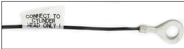
Figure 26 Coil Ground Wires
