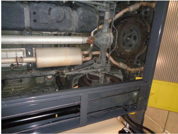
**Step 1.** Begin removal of the OE muffler by loosening the three clamps attaching the muffler to OE system. Disengage the hangers from the rubber insulators and remove the muffler. Do not discard or damage the rubber insulators as they will be used to install the new system.
