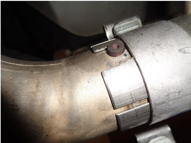
**Step 2:** To install the MagnaFlow Y-Pipe Assembly slide the inlet onto the OE outlet making sure to align the slot with the peg on the outlet pipe. Secure with the supplied 3.00" clamp.
