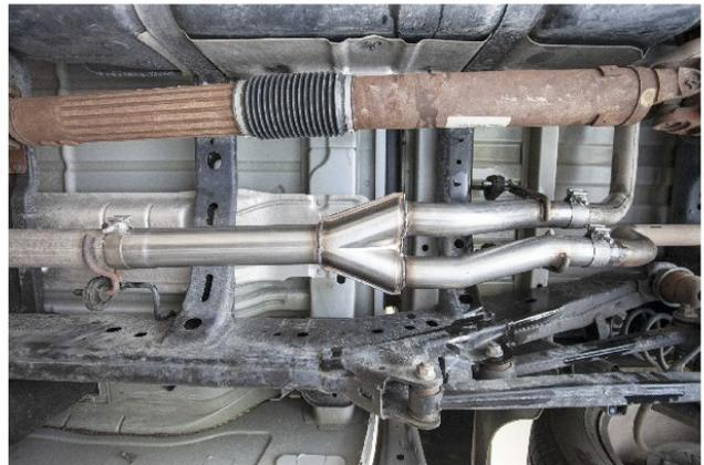
**Step 4:** Finish by fitting the OE tailpipes into the Y-Pipe Assembly by indexing the alignment pegs and securing with the supplied 2.25" clamps. Once a final position has been chosen for the new exhaust component, evenly tighten all clamps from front to rear using the torque specifications on page one of these instructions. Inspect all fasteners after 25-50 miles for operation and re-tighten if necessary.
