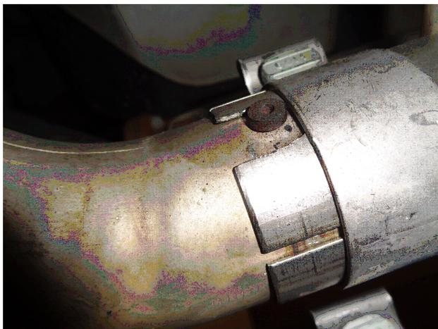
Step 2: To install the MagnaFlow Muffler Assembly slide the inlet onto the OE outlet making sure to align the slot with the peg on the outlet pipe. Secure with the supplied 3.50" clamp.
