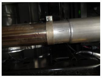
Step 2. Begin installation of the MagnaFlow system by attaching the Inlet Pipe to the outlet of the DPF using the supplied 4.50" clamp.
