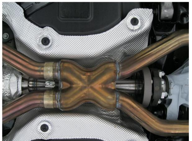
**Step 4.** Attach the X-Pipe Assembly to the Resonator Assemblies using the supplied 2.50" clamps.
