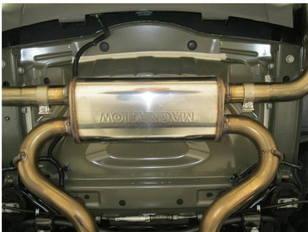
**Step 5.** Next install the Muffler Assembly to the X-Pipe Assembly using the supplied 2.50" Clamps and fit the hangers into the rubber insulators.
