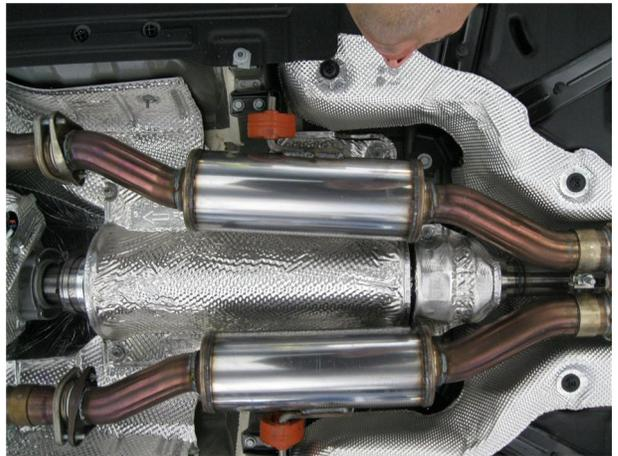
**Step 3.** Begin installation of the new Magnaflow system by using the supplied M10 bolts and OEM nuts to attach the Driver and Passenger Side Resonator Assemblies to the catalytic converter outlets.
