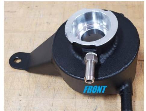
Figure 6 (PG Coolant Reservoir)
