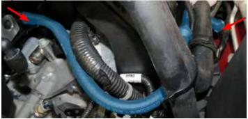
110. Connect the supplied EVAP hose to the hardline on the firewall at the rear passenger side of the manifold. Route the hose along the driver side of the manifold, beneath the coil wires, and connect it to the EVAP solenoid.
