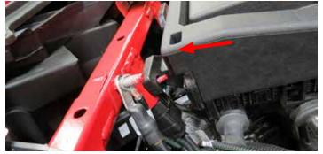
124. Route the EVAP connectors on the supplied water pump harness towards the EVAP solenoid. Install the water pump harness in-between the mating connectors on the EVAP solenoid and factory harness. TIP: Note connector orientation..
