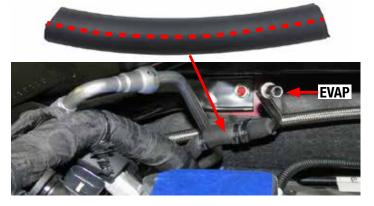
70. Connect the supplied fuel feed line to the hard line on the firewall and route it over towards the fuel adapter line. Secure the fuel line to the brake line with wire ties.
