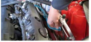
23. Unplug the MAP connector from the MAP sensor. Remove the MAP sensor from the manifold using a 10mm socket. This sensor will be reused later in the installation.
