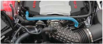
13. Using a hose clamp tool, remove the noise generator hose from the inlet elbow. Loosen the warm clamps securing the inlet elbow and remove the elbow.
