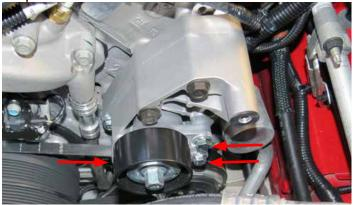
67. Install the larger grooved idler pulley to the FEAD bracket. Torque bolt to 22 ft-lbs.
