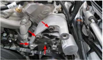
65. Position the ground strap behind the engine harness bracket and secure the engine harness to the cylinder head. Reconnect the engine harness.
