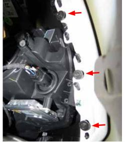
7. Disconnect the lamp and sensor harness located on the left side of the vehicle and carefully remove the fascia.
