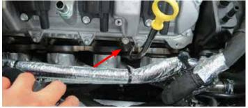
45. Remove five (5) bolts securing the passenger side exhaust manifold to the cylinder head. Carefully remove the exhaust manifold along with the dipstick. Discard the exhaust manifold gasket.
