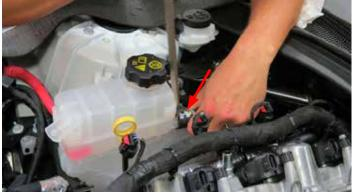
39. Using a deep 10mm socket, remove three (3) nuts securing the coolant reservoir tank. Remove reservoir and set aside.
