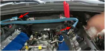
28. Remove oil cap. Using a Torx T30, remove the driver and passenger side coil covers. Replace oil cap to prevent debris from falling into the engine.
