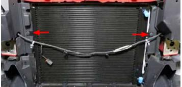
95. Secure the lower portion of the LTR to the air ducts using two (2) M6 x 16mm bolts and two (2) M6 locknuts from hardware Bag #2.
