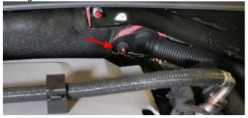
16. Remove the noise generator assembly by twisting the hose clockwise to unlock it from the firewall.
