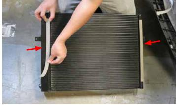
94. Position the LTR in front of the radiator assembly with the inlet barbs positioned on the driver side of the vehicle. Using the supplied push pins from hardware Bag# 2, secure the LTR to the radiator shrouds.
