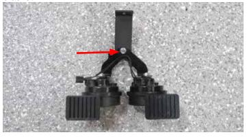
105. Install the horn assembly in the factory location using the factory bolt. Reconnect the horn connectors.
