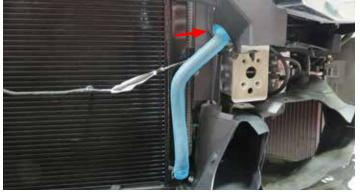
98. Using a 3/4" hose clamp from Bag #2, secure the LTR to Water Pump hose to the outlet barb of the water pump.
