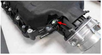
80. Apply O-ring lube to the O-ring on the EVAP solenoid and install EVAP port using the factory EVAP solenoid bolt.
