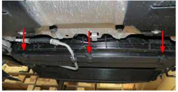
32. Disconnect the electric fan connector. Use a panel puller to detach the harness tree-clip from the fan shroud.
