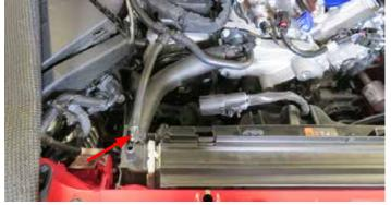
34. Using a hose clamp removal tool, detach the lower radiator hoses. 2017 model year Camaros only have drivers side lower hose. *NOTE: The clamps may not come off because of adhesive. Simply compress the clamp and pull the hose simultaneously.*
