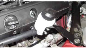
97. Using a 3/4" hose clamp from Bag #2, secure the LTR to Water Pump hose to the bottom LTR barb. Route the hose through the center opening of the radiator shroud.
