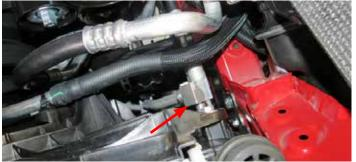
36. Using a panel puller, remove the coolant lines from the fan shroud.
