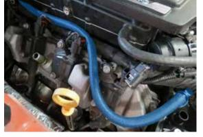
112. Connect the TMAP harness to the TMAP sensor located on the driver side of the manifold.
