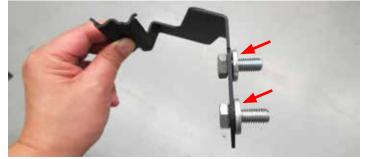
62. Using a 13mm socket, remove the ground strap from the engine block. Location is directly above the A/C compressor.
