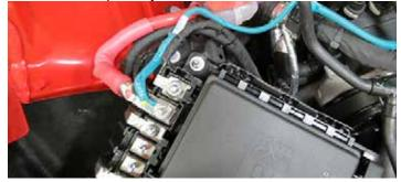
123. Remove the factory GROUND terminal nut attached to the chassis. Attached the GROUND connector on the water pump harness to the chassis ground and secure with the factory terminal nut. Remove the nuts securing the fuse box to the chassis. Gently remove the fuse box from the mounting studs and secure the relay to the mounting stud. Reinstall fuse box nuts.
