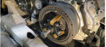
49. Apply white grease to the snout of the crank and to the inside of the balancer hub. Apply clean engine oil to the outside of the balancer hub.
