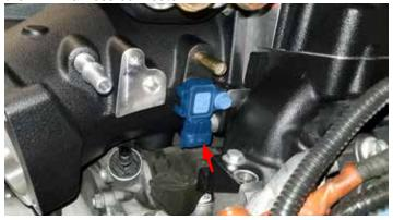
78. If equipped with the MAP adapter/hose assembly, install the long end of the nose, the short fitting end to the brake booster extender, and insert the factory MAP sensor and adapter into the short, straight hose end. Secure the sensor adapter with the suppplied hose clamp.
