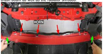
87. Using a 10mm wrench and a 13mm socket, remove ten (10) bolts, five (5) per side, securing the crash beam to the chassis. Remove push pin located underneath the crash guard on each side. Remove the crash guard.
