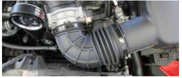
121. Using a razor blade or equivalent, remove the  $90^{\circ}$  fitting from the factory air inlet PCV hose. Connect the fitting to the supplied air inlet PCV and attach the straight quick connect to the air inlet and the  $90^{\circ}$  quick connect to the center PCV junction.
