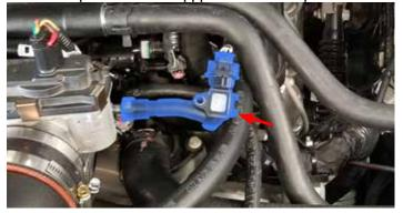
79. Using a 10mm socket, remove the EVAP solenoid from the stock manifold. Inspect the O-ring gasket and replace if needed.
