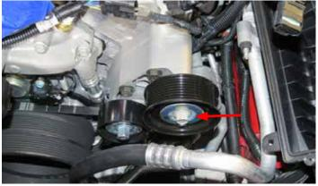
68. Install the smooth idler pulley to the upper water pump provision and the smaller grooved idler to the lower water pump provision. Torque both bolts to 22 ft-lbs.
