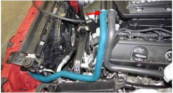
101. Using two (2) 3/4" hose clamps from hardware Bag #2, secure the Surge Tank to Manifold hose to the surge tank and rear water cross over barb.
