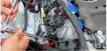
42. Disconnect the passenger side spark plug wires from the coil packs.
