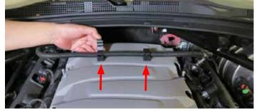
19. Using a deep 10mm socket, remove four (4) bolts securing the manifold cover. Unplug MAP sensor, and cut ties holding the harness to the intake. Do NOT damage the harness.
