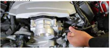
18. Unclip the fuel line from the top of the manifold.
