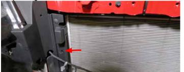
92. Using a panel puller, remove both inner push pins securing the right and left air ducts.
