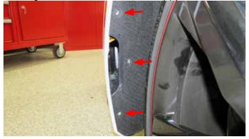
5. Use a 7mm socket to remove six (6) screws securing the corner of the fascia to the fender; three (3) per side.
