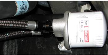
10. Install the oil filter on the remote oil filter adapter.
