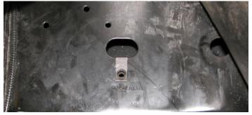
2. Hold the spacer perpendicular to the frame rail and align the lower hole with the J-nut then use a hole punch to mark the location of the upper hole.
