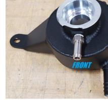
Figure 6 (PG Coolant Reservoir)
