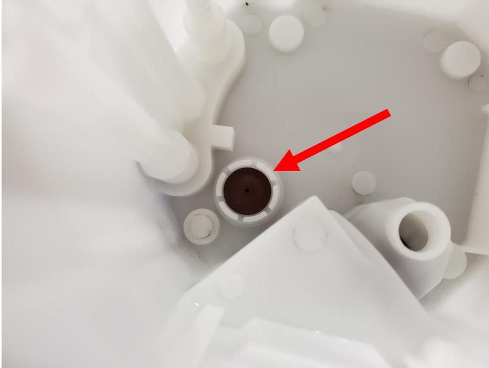
6 – Install the supplied smaller convoluted hose onto the venturi jet nipple inside the bucket, secure with the 8.5mm hose clamp.
