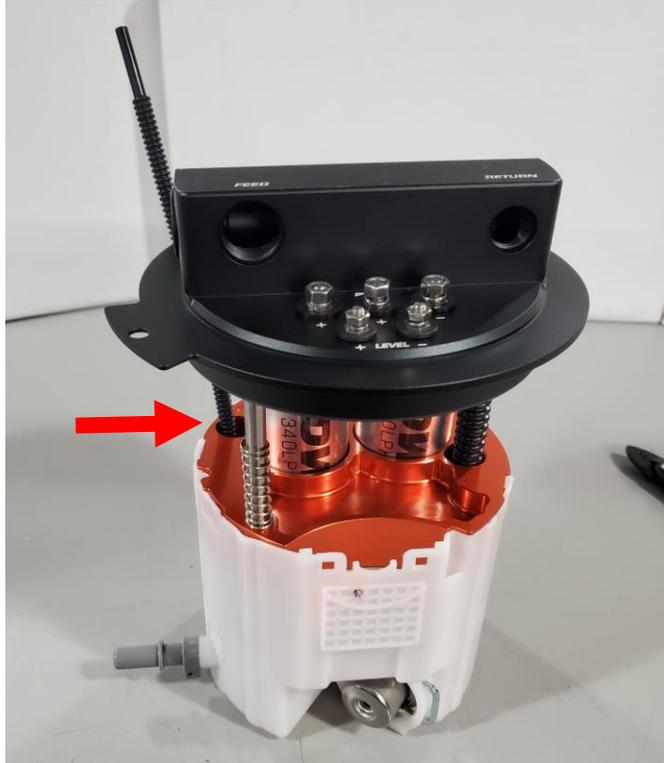
8 – Attach the remaining smaller 1/8-inch end of the venturi hose to the 1/8-inch hose barb fitting on the underside of the hat, and secure with the provided 6mm hose clamp.
