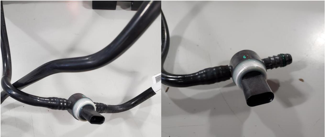
15 – Locate the adapter fittings and included O-rings. Remove any factory O-rings from the fuel pressure sensor. Install the supplied O-rings into the groove the OE O-rings were in, and the remaining two onto the very ends of the barbs against the sensor.
