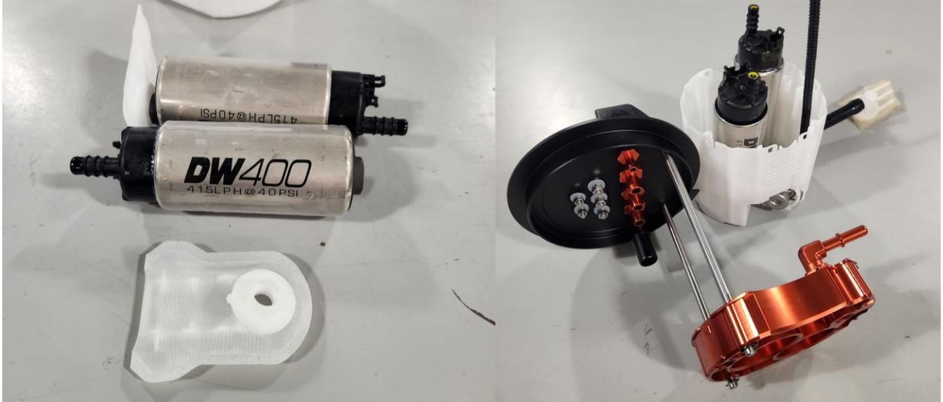
6 – Locate the remaining convoluted hoses, you should have three 10-inch long 3/8" hoses and one 10-inch long 1/4" hose remaining. Attach these hoses to the barbs on the bottom side of the X2 top hat, secure each one with the appropriate clamp.
